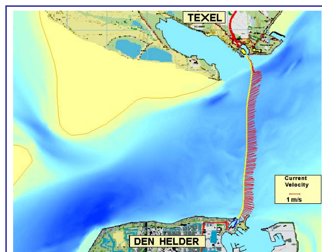
Figure 3-17: Example of a real-time display of current vectors along the ferry track between the island of Texel and Den Helder as typically displayed in the passenger area.
