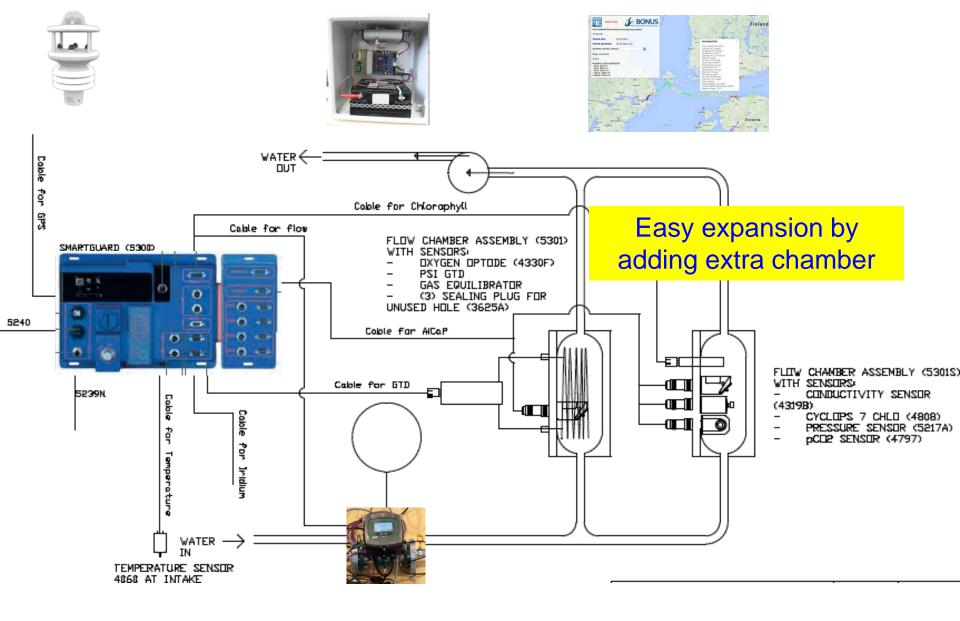
Modular system based off the shelf standard components
