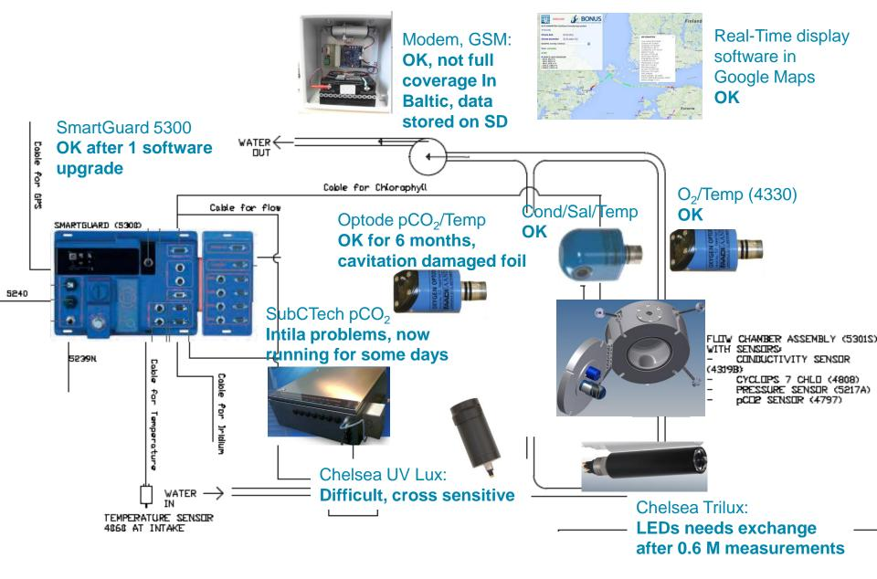
Sensor experience from Romantika, installed June 2013, running at 1 minute interval, about 1.1 Million measurements
