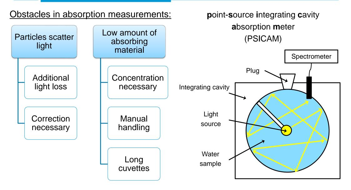
**<u>Aim</u>**: Adapting the PSICAM approach for flow-through operation
